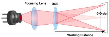
Laser diodes are the most common light source to be used with diffractive optical elements, but other laser light sources may also be used.
